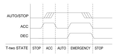
Diagram 1: AUTO/STOP and REEL SELECTION command functions
